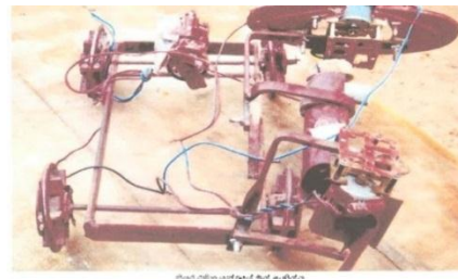
Framework of Paddy Field paring machine
