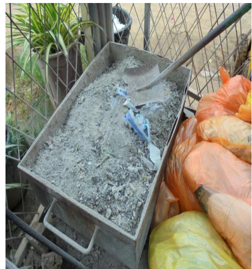
Photo: Presence of unburnt waste in the ashes disposed through the Incinerator installed at the Polonnaruwa Hospital.
