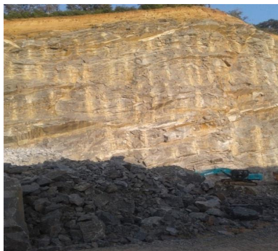
Diagram 29- Even though the mining should have been done from 10 to 10 meters under level basis, mining has been done at a slope of 90 degrees with the height of 30 meters.
