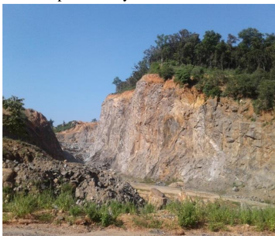
Diagram 29- Even though the mining should have been done from 10 to 10 meters under level basis, mining has been done at a slope of 90 degrees with the height of 30 meters.
